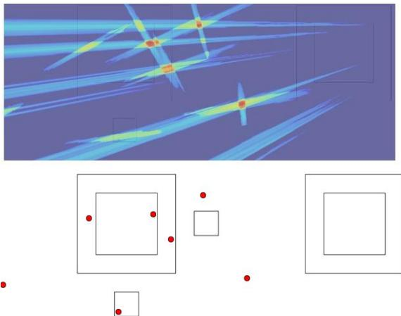
Fig. 5. Detection results for multiple people detection using the homography constraint. The top image show the accumulation result, and the bottom image shows the location of the detected people from the computation of local maxima [16].
