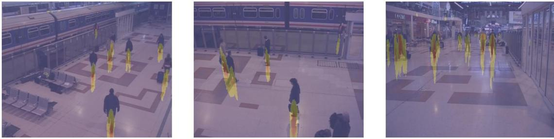
Fig. 4. Results of background subtraction superposed on top of the original images of 3 cameras [16].
