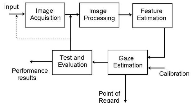
**Figure 3. Block Diagram of an EGT Device**
