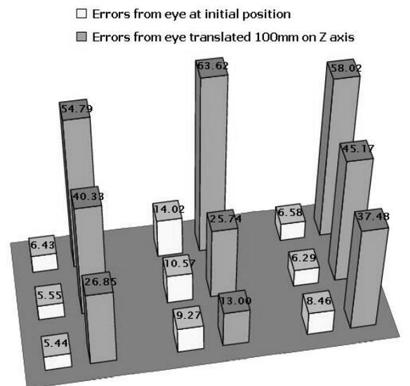
**Figure 6. Average screen grid errors (in mm) to eye at  $P_0$  and at  $(0, 270, 700)$ .**
