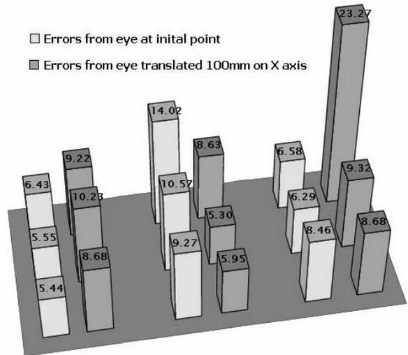
**Figure 5. Average screen grid errors (in mm) to eye at  $P_0$  and at  $(-100, 270, 600)$ .**
