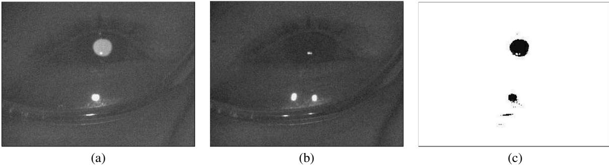
**Figure 2. Bright (a) and dark (b) pupil images resulting from on and off axis illumination. (c) shows the difference image of the dark image subtracted from the bright.**
