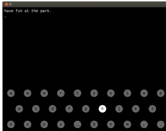
**Figure 1:** Virtual keyboard used in the experiment. The background has zero brightness, the keys' background have brightness 50%, and highlighted keys have brightness 100%.
