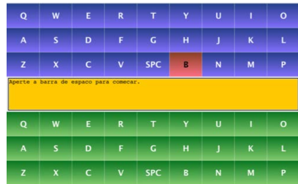
Figure 1. Virtual keyboard for eye typing based in the Context Switching paradigm, image reproduced from Morimoto and Amir.
