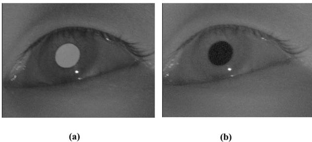
Fig. 2. (a) Bright and (b) dark pupil images. The glints, or corneal reflections, from the on and off-axis light sources can be easily identified as the bright regions in the iris.
