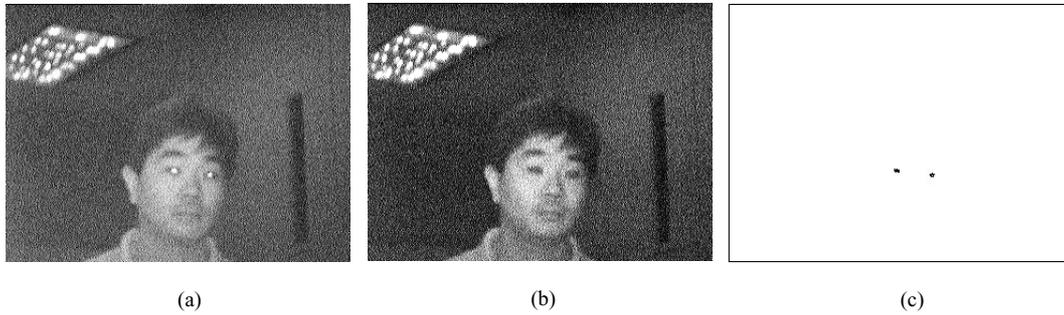
Fig. 4. (a) Bright and (b) dark pupil images; (c) shows the pupils detected using a temporal support of four frames.
