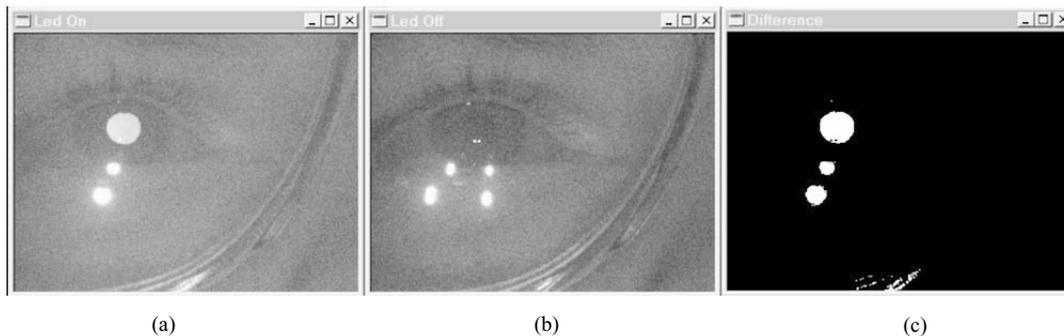
Fig. 5. (a) Bright and (b) dark pupil images of a person wearing glasses. (c) shows the pupils candidates. The false candidates are caused by the reflections of the on-axis light source from the back and front surfaces of the glasses.
