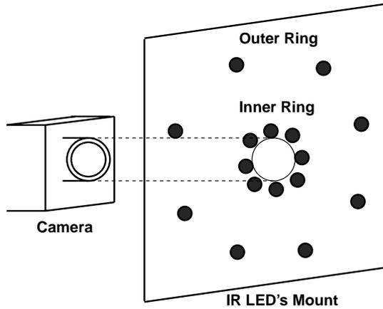
Fig. 1. Camera and infrared illuminators.
