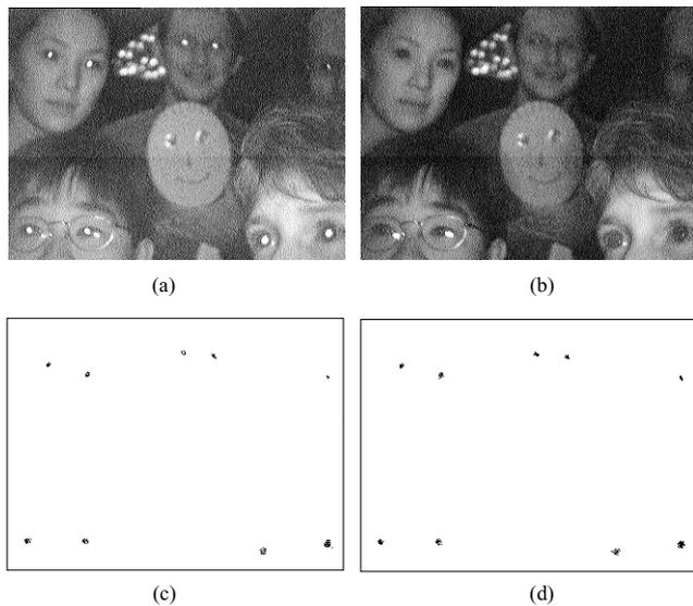
Fig. 3. (a) Bright and (b) dark pupil images. (c) and (d) show the pupils detected from subtraction and thresholding using the corresponding previous frames, after erosion.
