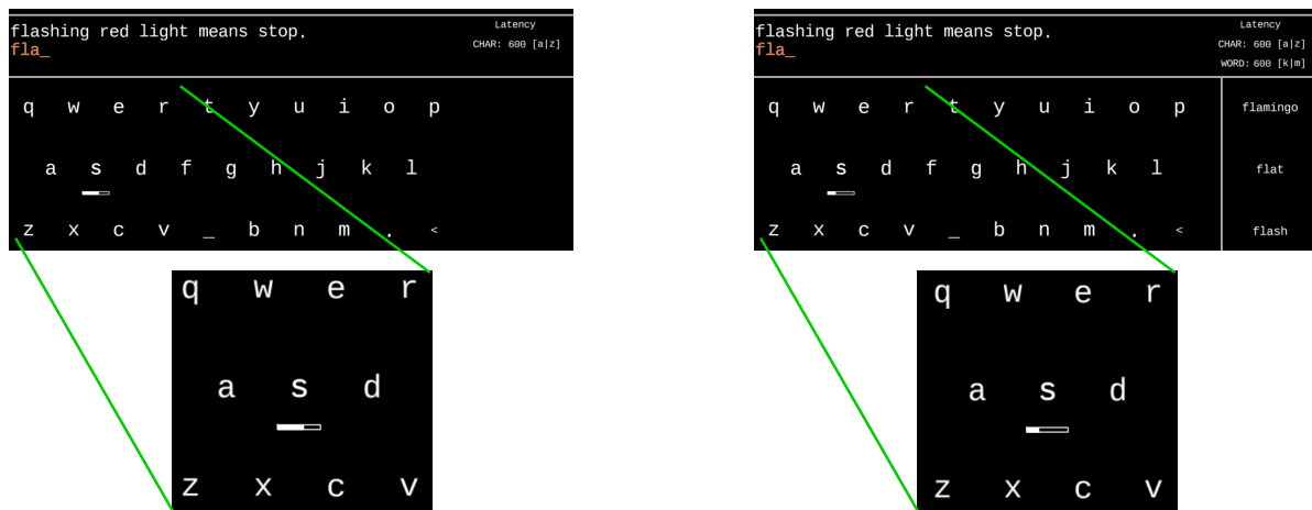
Figure 1. Dwell-time based virtual keyboards without word prediction (left) and with word prediction list (right). The 's' key has the user focus, indicated by the progress bar below the key.
