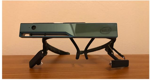
**Figure 5:** The Pupil binocular eye tracker coupled with an Intel Realsense R200 camera used as head-mounted setup.
