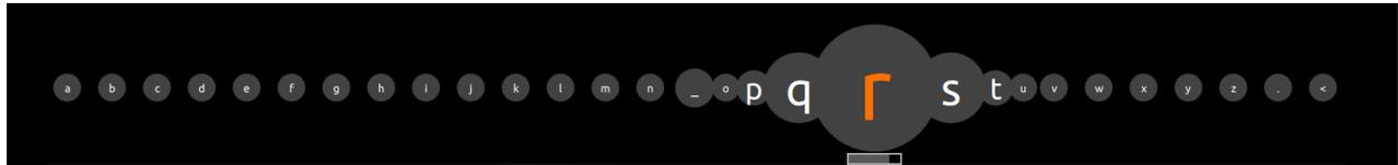
Figure 1: Dense single line keyboard layout with dynamic expanding targets. Keys are selected by dwelling.
