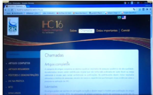
(b) Screen image after the homography transformation. Note that all background has been removed and the screen image is undistorted.
