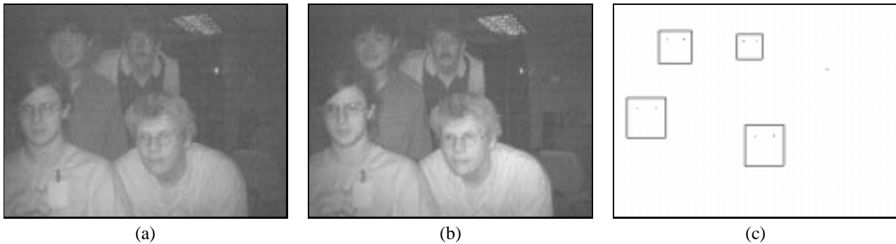
Figure 4. (a) Bright and (b) dark pupil images. (c) Difference and detected faces.
