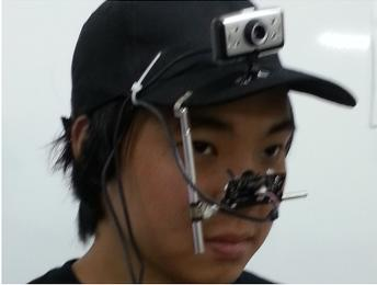
**Figure 2:** Low cost wearable head mounted eye tracker.
